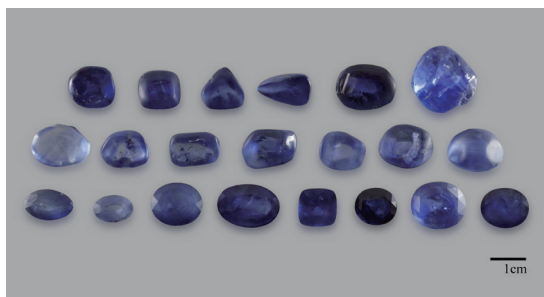
Fig. 5 Another set of previously heated sapphire samples (left) showing slight loss of colour in some samples and slightly improved colour and clarity in others after heat and pressure treatment (right). Photo by P. Ounorn
