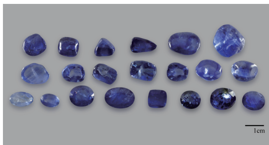
Fig. 5 Another set of previously heated sapphire samples (left) showing slight loss of colour in some samples and slightly improved colour and clarity in others after heat and pressure treatment (right). Photo by P. Ounorn
